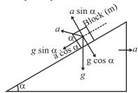
So, from the above free body diagram (FBD), Acceleration of body sliding up over inclined plane.  $a = g \sin \alpha + a \cos \alpha$  ...(i) Acceleration of body sliding down over a rough inclined plane
