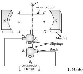
**Working:** When a coil is rotated in magnetic field, an emf is induced in the coil. The coil may be rotated by water energy, steam energy or oil energy. Let at any instant magnetic flux through armature coil,
