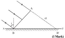
Let in time 't' the secondary wavelets reaches B' covering a distance ct. Similarly from each point on primary wavefront AB. Secondary wavelets start growing with the speed 'c'. To find reflected wavefront after time 't', let us draw a sphere of radius 'ct' taking 'B' as center and now a tangent is drawn from B' on the sphere the tangent B'A' represents reflected wavefront after time t.
