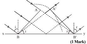
For every point on wavefront AB a corresponding point lie on the reflected wavefront A'B'.
