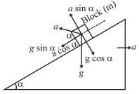
So, from the above free body diagram (FBD), Acceleration of body sliding up over inclined plane.
